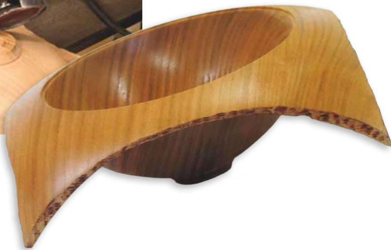
◀ Pic.35 Remove as much as you can on the lathe and take away the remaining timber using a carving or sanding tool - the Proxxon mini angle grinder with a sanding pad is perfect for this
